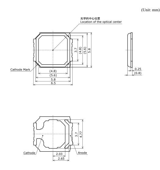
Figure 1. Outline dimensions of the NFMW48xAR Series LEDs (excerpted from the specification)
