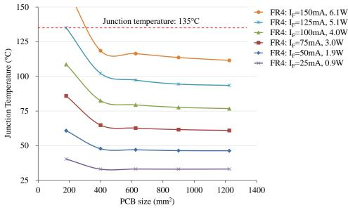
Figure 6. Results of the evaluation using the FR4 substrate
