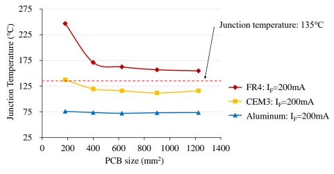
Figure 5. Evaluation results per PCB material
